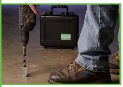
moisture condition of the floor is relative humidity (RH) testing using in situ probes, ASTM F2170. A series of test holes are drilled into the slab and a small probe is placed into the hole where it is allowed to equilibrate with the slab before readings are taken. Research has found that placing the probe internally, at a depth of 40% of the slab's total thickness (if drying one side),
