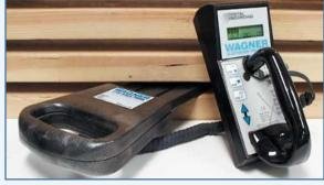
With a Spare Stack Probe Head in your stock, you can NOW eliminate the need and shipping expense of sending the whole Stack Probe in to Wagner. All you have to do is remove the Stack Probe Sensor Head, install Spare Probe Head and send just the damaged Probe Head in for repair/eval (see back of this card for the replacement procedure).
